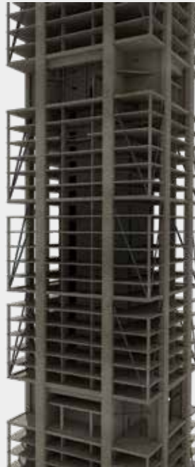
Fig. 14: Left: A corner hang is installed. Right: A massing model shows the hangers
