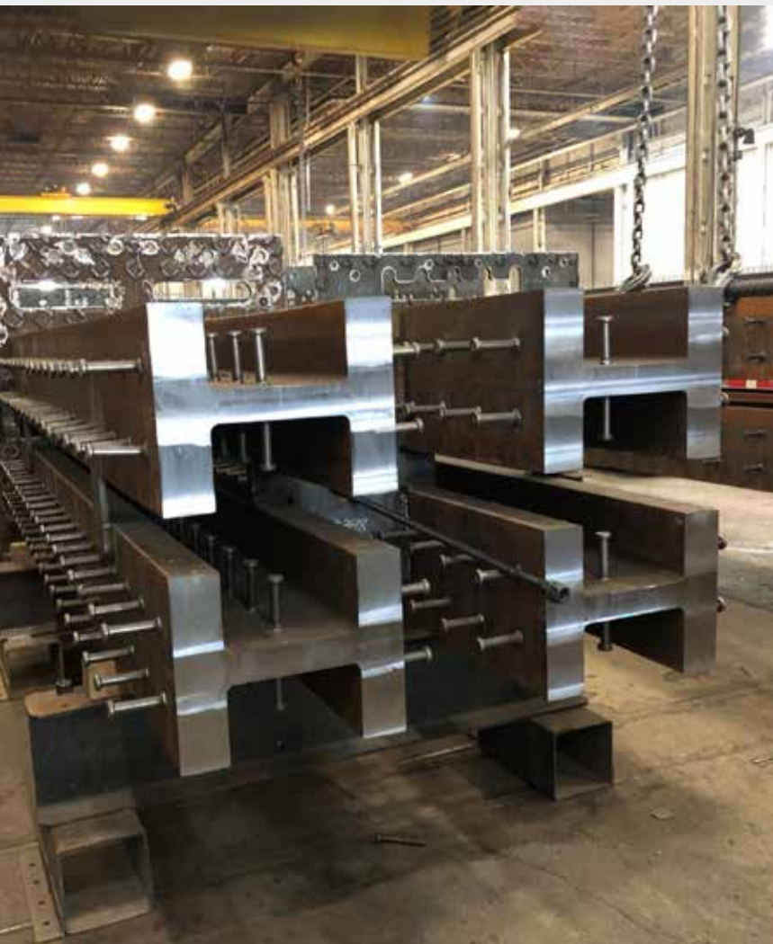
Fig. 7: Composite Mega Column in the fabrication shop
